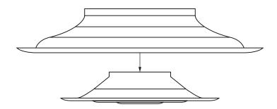
**STEP 4:** Align and fasten the outer cone's inlet to the round hard duct. Inlet collar or sheet metal band (by others) can be used to fasten the inlet to the hard duct.
