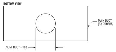
**STEP 2:** Align the DRF flange with the round opening in the main duct. Ensure that the hole in the main duct aligns with the inside of the DRF. Screw the DRF into the main duct using self-tapping screws.
