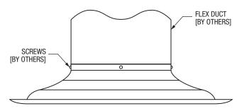
**STEP 3:** Lift the diffuser to the appropriate height and screw hanger straps to the diffuser's neck or outer cone. Ensure the screws will not be visible once the inner core is reattached.
