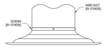
STEP 3: Once the diffuser is securely fastened, reattach inner core assembly to the outer cone (see Page 3).
