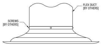
**STEP 4:** Lift the diffuser to the appropriate height and screw hanger straps to the diffuser's neck or outer cone. Ensure the screws will not be visible once the inner core is reattached.
