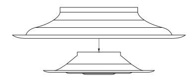
**STEP 2:** Align and fasten the outer cone's inlet to the round hard duct. Inlet collar or sheet metal band (by others) can be used to fasten the inlet to the hard duct.
