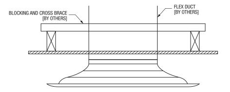
STEP 8: Align and fasten the outer cone's inlet to the duct. Inlet collar or sheet metal band (by others) can be used to fasten the inlet to the duct.
