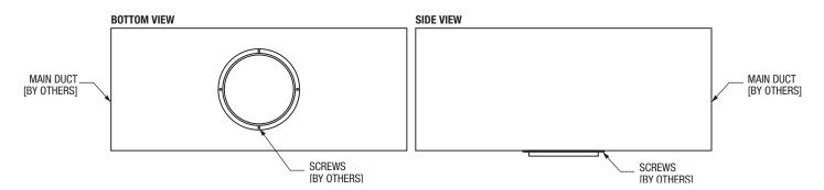
**STEP 3:** Once the DRF is securely in fastened, align the hard round duct around the DRF and screw the hard ducting into the DRF using self-tapping screws.
