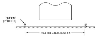
**STEP 4:** Push the PR in the opening so that the bottom flange of the PR comes in contact with the ceiling. Once in place, screw the PR into blocking using self-tapping screws.
