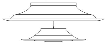
STEP 3: Align and fasten the outer cone's inlet to the flex duct. Inlet collar or sheet metal band (by others) can be used to fasten the inlet to the duct.
